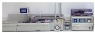
high throughput setup with blood addition pump and ProfiClave Agar preparator
